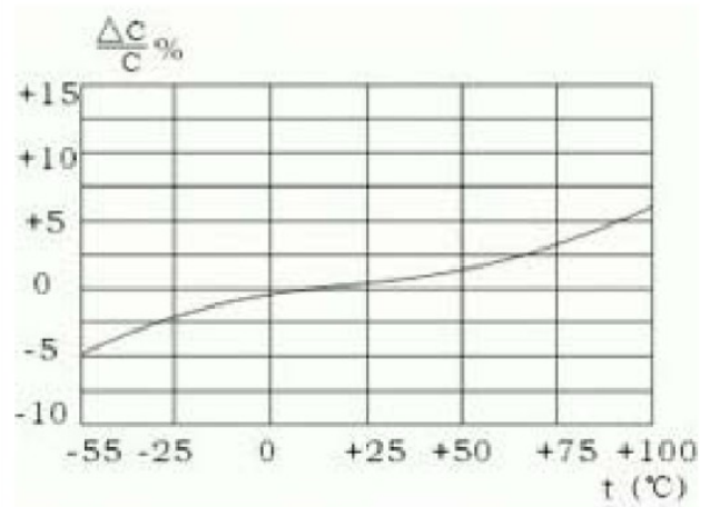
Capacitance vs. temperature (1KHZ)
